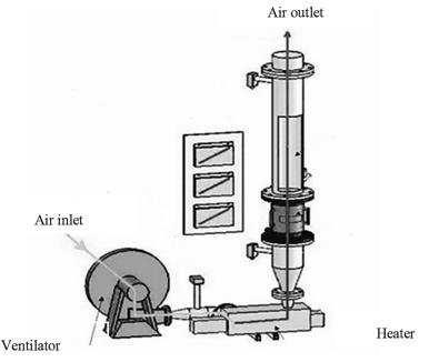
Figure 1. Pilot plant drying by fluidization (Deltalab-France)
