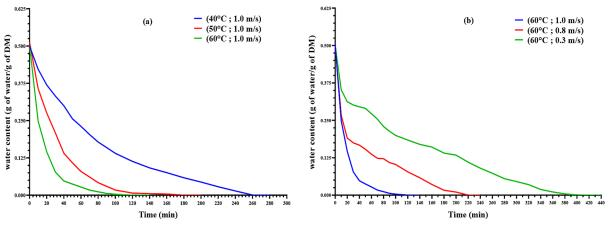
**Figure 3.** Effect of drying air temperature and speed on myrtle leaves drying kinetic: (a) at a variable temperature and fixed speed (1 m/s); (b) at a variable speed and fixed Temperature (60 °C)
